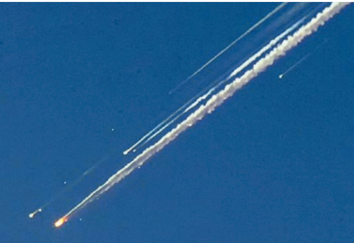
According to CAIB, destruction of the crew module took place over a period of 24 seconds, beginning at an altitude of approximately 42,672m and ending at 32,000m. Credits: NASA
